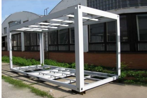
Hình 1. 1. Khung container ( nguồn : https://xuatnhapkhauthucte.com/cau-truc-cua-container/ )
