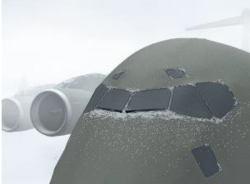
Figure 14.5 , Frost on Exposed Surfaces of Parked Aircraft.
