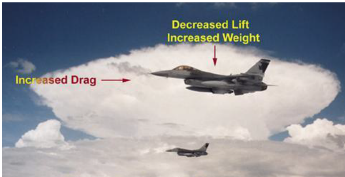
Figure 14.6, Effects of Icing are Cumulative Causing Stall Speed to Increase.
