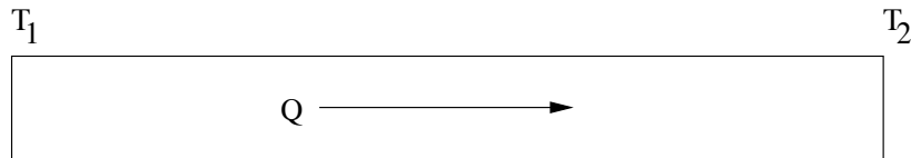
Figure 7.1: A temperature gradient in a metal bar as an example of a nonequilibrium system. Here Q is the flow of heat from the higher temperature T_1 to the lower temperature T_2 .
