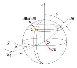
At the centre of the sphere the electric field due to the volume charge will be zero because the contribution of a volume element located at  $\mathbf{r}'$  will be exactly cancelled by that of an equivalent volume element at  $-\mathbf{r}'$ , so we only need to consider the surface charge.
