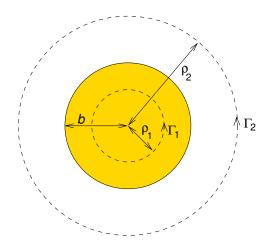
We define the z axis to correspond the axis of the wire, and point out of the screen/page. Then assuming the current density is constant inside the wire
