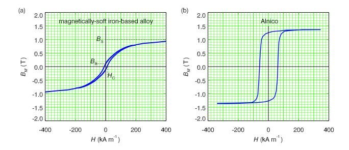
Grid lines have been drawn over the hysteresis plots above. The area of the upper half of the hysteresis loop (for positive  $B_M$ ) is identical to that of the lower half. Read off the (horizontal) "widths" in H at "heights"  $B_M = 0, 0.1, 0.2, \ldots$  (T). The approximate values are tabulated below.
