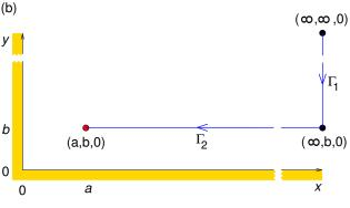
(b) We first calculate the force on charge +q at its final position due to the induced surface charge on the conductor as if it were due instead to the image charges as in part (a) of diagram above,
