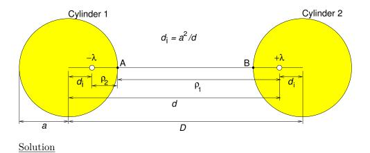
The potential at A (and conductor 1 surface) due to the image line charges is,
