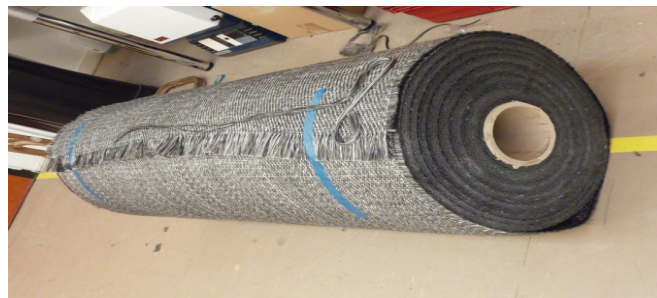
Figure 1.21 A roll of PP-GF Twintex fabric
