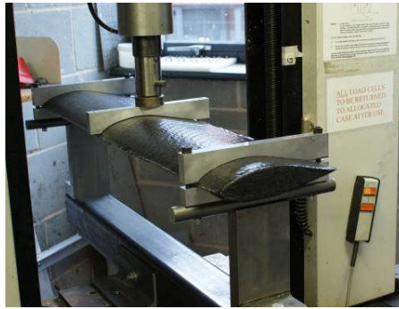
Figure 5.7 Picture of 3-P bending test setup with a span of 850 mm (source: Brown & Brooks 2009)
