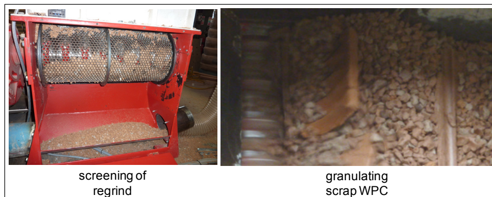
Figure 2.31 Photographs of a WPC granulator
