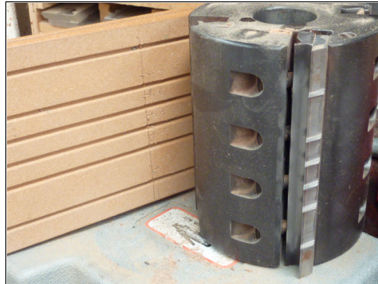
Figure 2.30 The rotary profile/moulding cutter
