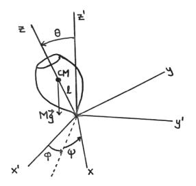
We consider a heavy symmetric top spinning about its principal axis in the gravitational field. The gravitational acceleration is g. One point on the symmetry axis is fixed. The coordinate system x'y'z' is now taken to be fixed in space so that  $g = -g\hat{z}'$ , whereas xyz lies fixed in the body such that  $\hat{z}$  is the symmetry axis. The geometrical symmetry implies that
