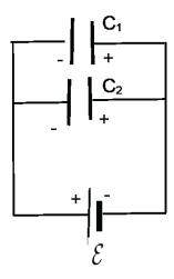
We consider two capacitors  $C_1$  and  $C_2$  connected in parallel, as shown. The two capacitors have the same voltage drop  $\mathcal{E}=V=V_1=V_2$  so that the charges on the two capacitors follow  $Q_1=C_1V$  and  $Q_2=C_2V$ . The total charge  $Q=Q_1+Q_2$  determines the equivalent capacitance:  $Q=Q_1+Q_2=C_1V+C_2V$ , or
