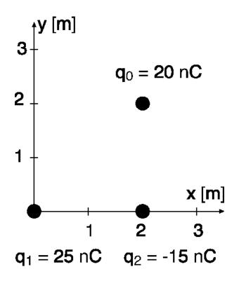
**Example 5:** Two charges  $q_1$  and  $q_2$  are placed on the xy-plane as shown. **a)** Calculate the electric potential at the location of the charge  $q_0$ . **b)** Calculate the electrostatic potential energy of the charge  $q_0$  and **c)** interpret your result.
