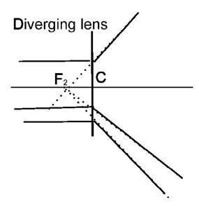
The incoming rays of an object (infinitely) far away are refracted in a *diverging* lens such that they diverge: their continuation backwards intersect at the focal point  $F_2$ : the distance between the center of the lens and the focal point is the focal length f. The focal point  $F_2$  is in front of the lens and we use the convention
