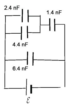
**Example 9:** Four capacitor  $C_1=2.4\,\mathrm{nF}$ ,  $C_2=4.4\,\mathrm{nF}$ ,  $C_3=1.4\,\mathrm{nF}$ , and  $C_4=6.4\,\mathrm{nF}$  are connected as shown. a) Find the equivalent capacitance. b) If  $\mathcal{E}=12\,\mathrm{V}$ , find the voltages across each capacitor.
