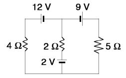
Example 4: The circuit consists of three batteries and three resistors as shown. a) Label the circuit and write down Kirchoff's loop and junction rules for the circuit. b) Find all the currents in the circuit! c) What is the total power dissipated in the circuit? d) What is the total power delivered by the three batteries in the circuit?
