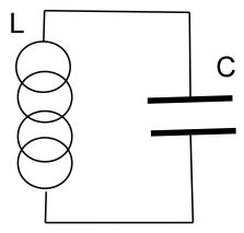
**Example 6**: A capacitor with  $C=4.6\mathrm{nF}$  is connected to an inductance with  $L=3.2\,\mathrm{mH}$ . a) Show that the charge (and thus the current) in the cicuit exhibits oscillatory time dependence. b) Determine the period of oscillation. c) If the capacitor is fully charged at time t=0 with  $Q_0=1.3\,\mathrm{pC}$ , find the maximum value of the current in the circuit.
