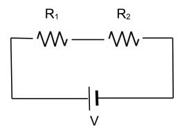
We consider two resistors  $R_1$  and  $R_2$  in series, as shown. The current through the two resistors is the same as the current through the battery I. The voltage drops across the two resistors  $V_1=R_1I$  and  $V_2=R_2I$  add up to the voltage of the battery:  $V=V_1+V_2$ . We introduce the equivalent resistance  $V=R_{\rm eq}I$  and find
