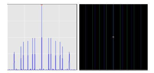
When the number N of slits is increased, the number of minima and maxima increases. The intensity of some minima does not change with N [principal maxima], whereas the intensity of great many maxima decreases as N increases [secondary maxima]. When N becomes of the order of hundred or thousand, the secondary minima can no longer be observed, and only the primary maxima 'survive.' This arrangement is called a diffraction grating. The angles of the m-th order principal maxima is given by
