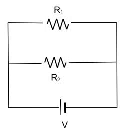
We consider two resistors  $R_1$  and  $R_2$  in parallel, as shown. The potential drops across the two resistors  $V_1$  and  $V_2$  is equal to the voltage of the battery:  $V=V_1=V_2$ . Since  $I_1=V/R_1$  and  $I_2=V/R_2$  are the currents through the resistors  $R_1$  and  $R_2$ , respectively, the current through the battery is the sum  $I=I_1+I_2$ . We introduce the equivalent resistance  $I=V/R_{\rm eq}$  and find
