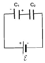
We consider two capacitors  $C_1$  and  $C_2$  connected in series, as shown. The charge on both capacitors are the same  $Q_1=Q_2=Q$ . We note that the voltage drops across the two capacitors add up to the electromotive force  $\mathcal{E}=V=V_1+V_2$ . Since  $V_1=Q/C_1$  and  $V_2=Q/C_2$ , we write  $V=Q/C_{\rm eq}=Q/C_1+Q/C_2$ , or
