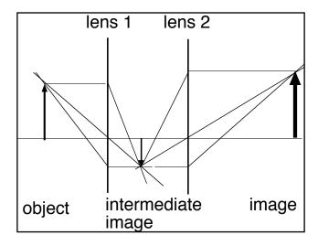
Both lenses are converging. The focal lengths are
