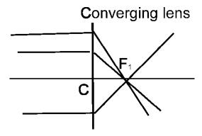
The incoming rays of an object (infinitely) far away are refracted in a *converging* lens such that they intersect at the focal point  $F_1$ : the distance between the center of the lens and the focal point is the focal length f. The focal point  $F_1$  is behind the lens and we use the convention
