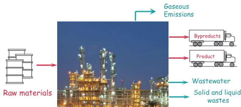
Figure 1.3 Metabolism of an industry. Materials that are not converted into products or useful byproducts become wastes or emissions that are contaminated by reactants, impurities in reactants, useless byproducts, solvents, catalysts, and lost products. (Photo credit: freedigitalphotos / supakitmod)
