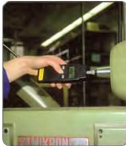
**Figure 5.9** Digital Tachometer
