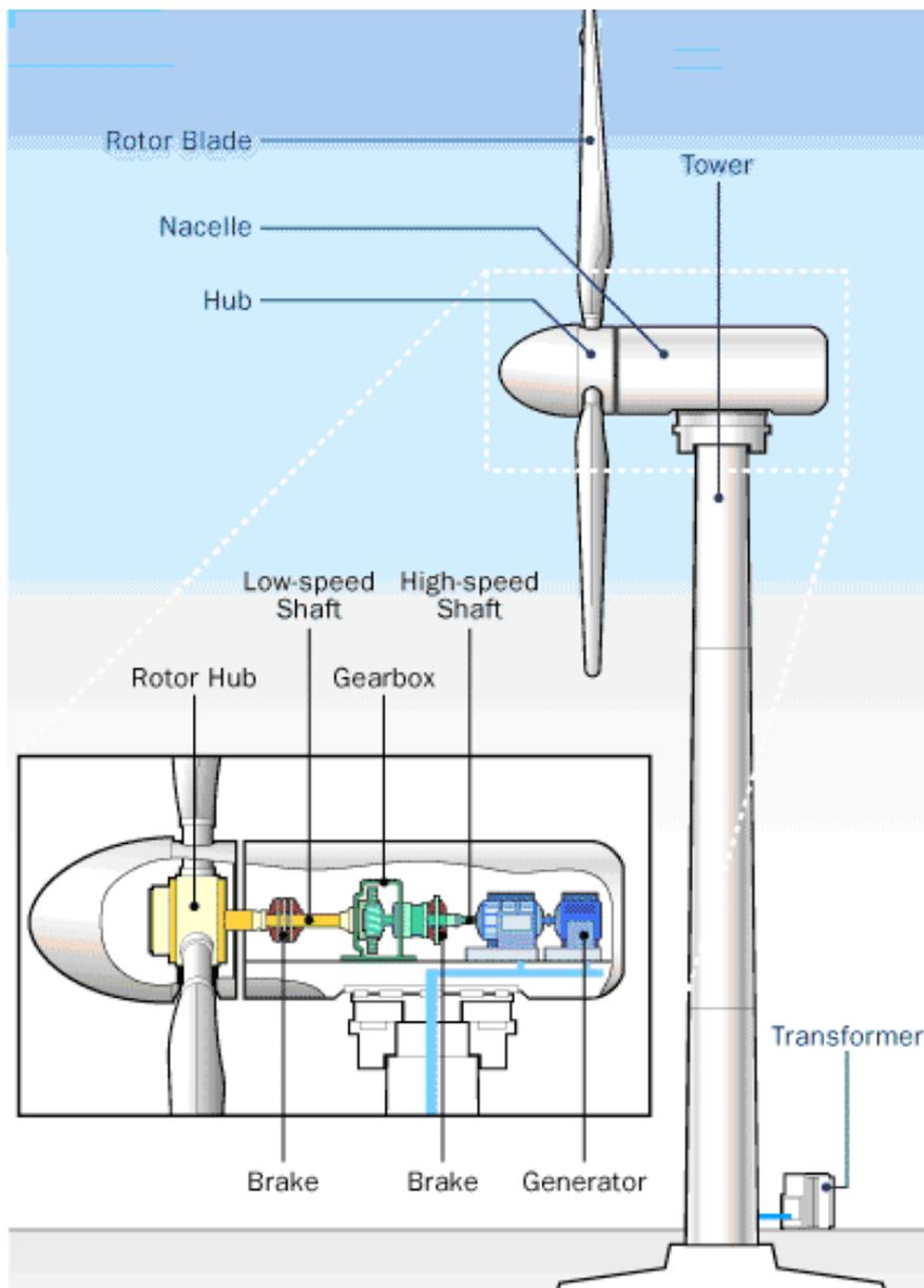
**Figure 1.1** Energy conversions in a typical Wind Turbine.
