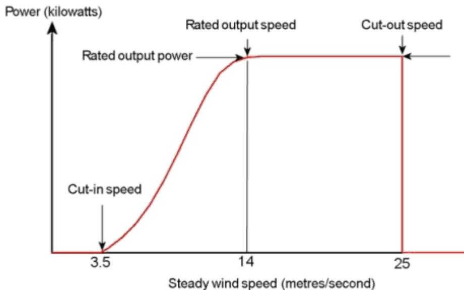
**Figure 5.13** Wind speeds for a wind turbine
