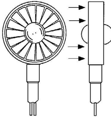
**Figure 5.6** Vane Anemometer
