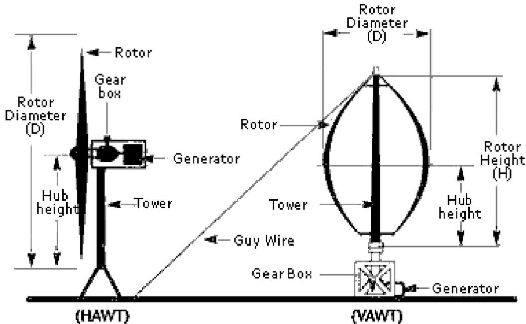
**Figure 4.2** Wind Turbine components
