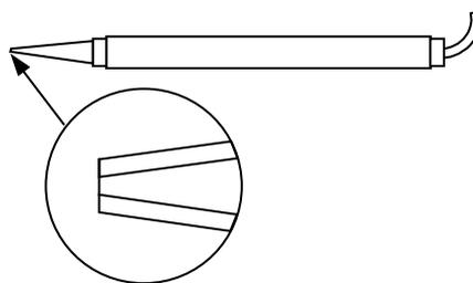
**Figure 5.7** Hot-Wire Anemometer
