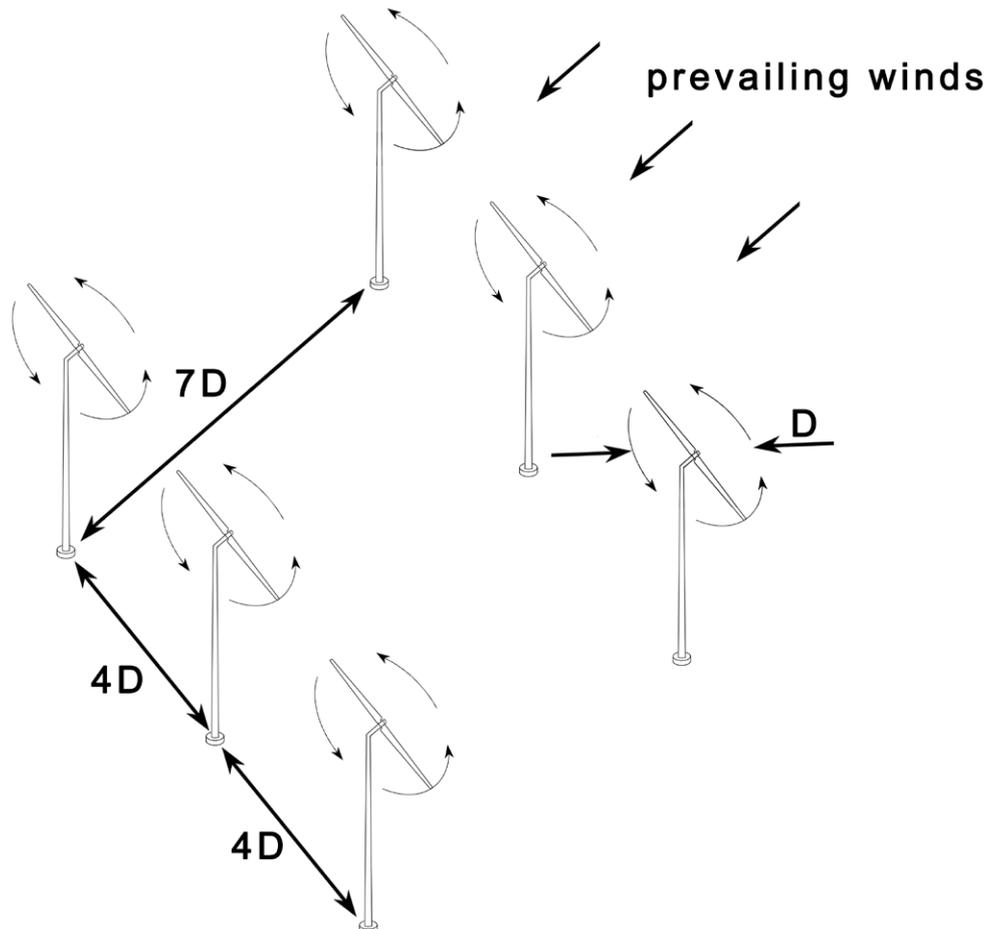
**Figure 2.3** Wind farm optimal placement
