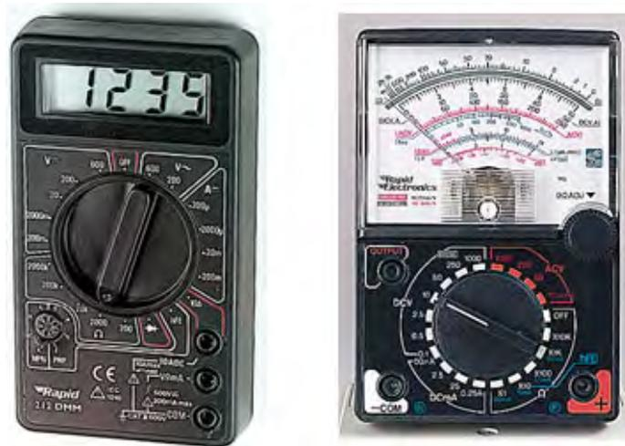
Figure 5.3 Digital and Analog Multimeters
