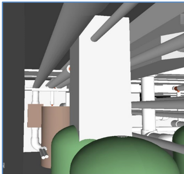
Figure 9.9: M+E water tanks clashing with structural concrete column highlighted by clash detection
