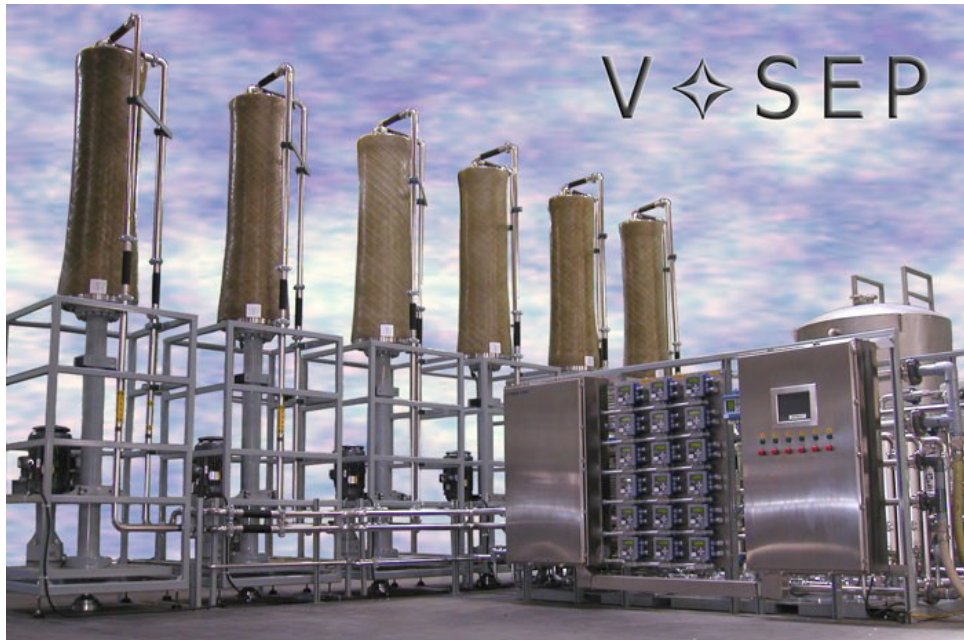
Fig 23. Industrial VSEP modules with 150 m 2 of membranes
