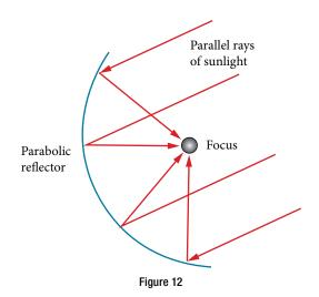
Parabolic mirrors have the ability to focus the sun's energy to a single point, raising the temperature hundreds of degrees in a matter of seconds. Thus, parabolic mirrors are featured in many low-cost, energy efficient solar products, such as solar cookers, solar heaters, and even travel-sized fire starters.
