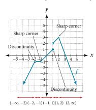
Figure 17 Five intervals where the function is differentiable
