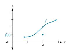
Figure 7 Conditions 1 and 2 are both satisfied. Condition 3 fails.
