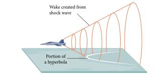
Figure 1 A shock wave intersecting the ground forms a portion of a conic and results in a sonic boom.
