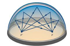
Figure 12 Sound waves are reflected between foci in an elliptical room, called a whispering chamber.
